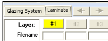
Figure 1-2. Click on the Laminate tab to start constructing a laminate.
