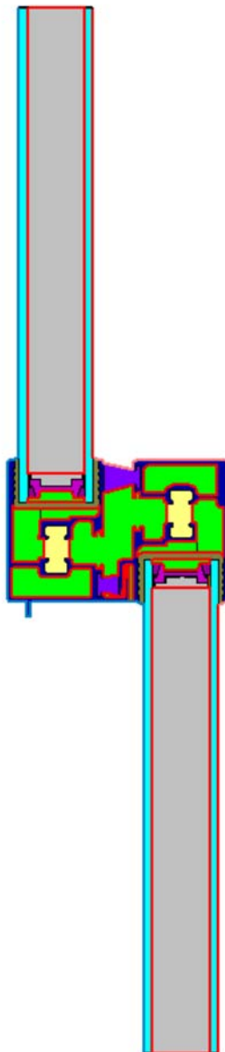
Figure 8-11. Red boundary conditions will appear inside the glazing system when the Condensation Resistance feature is activated.
