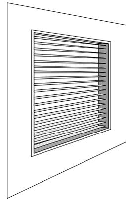
*An exterior shade screen fits neatly within window framing, a bit away from the glass. Design for easy removal for cleaning.*
